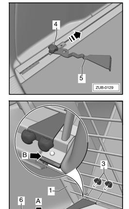
Insert one screw -6- into each of the holes in the retainer
